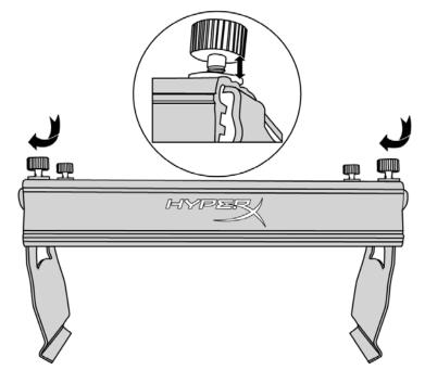
Step #2: To assemble the HyperX fan, secure the two side brackets with the four thumb screws / washers. Do not tighten the screws completely!
