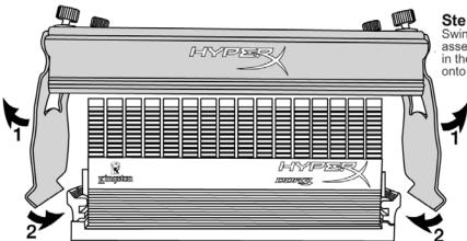
Step #3: Swing the retaining brackets open and slide the assembly over the HyperX modules as shown in the illustration. Rest the base of the brackets onto the memory socket lock tabs.
